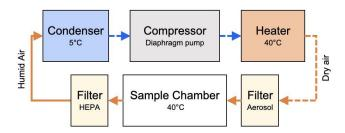
Evapinator consists primarily of an Arduino Uno, aluminum heating and condensing blocks, thermoelectric coolers (TECs), air filters, and a 3D-printed PLA sample chamber. All components were available for purchase either on Amazon.com or Digikey.com. The sample chamber was printed on the Bambu X1 printer using commonly available PLA filament. The aluminum heat block was milled from stock. The remaining mounting was performed with laser-cut acrylic.
