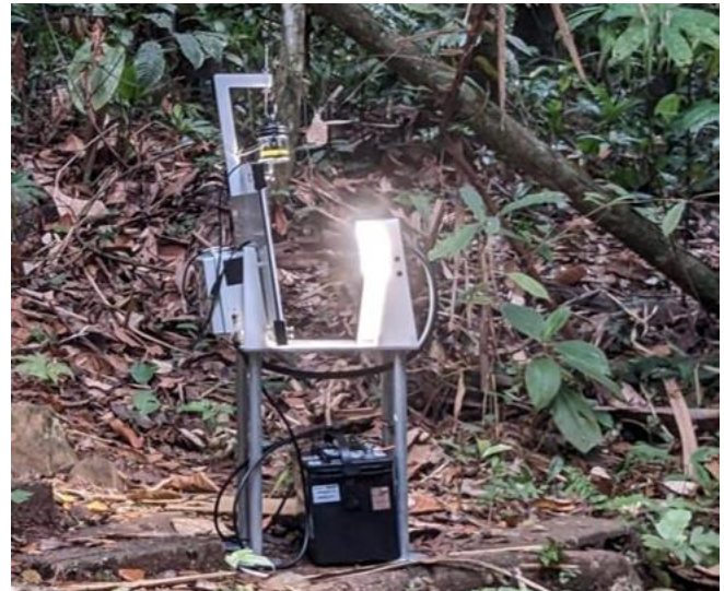
Fig. 1. Existing research-grade AMI system for automated monitoring of insects. It has a light to attract insects (top), a camera to take photos (right), and a big battery (bottom). Dozens of AMI system have been deployed around the world, but they are expensive and bulky. © UKCEH.
