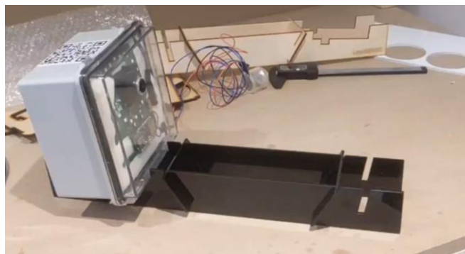
Fig. 3. Prototype in its weather-proof housing on a laser-cut stand. © Tom August, UKCEH.
