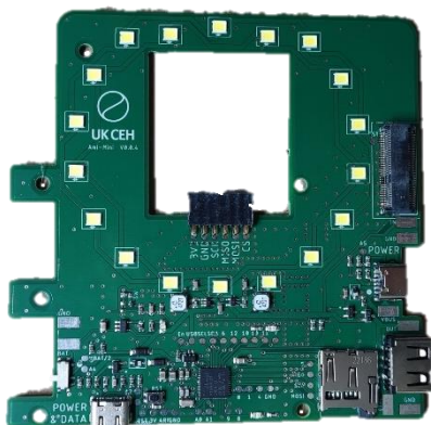
Fig. 2. Printed circuit board with cut-out for camera surrounded by light emitting diodes (LEDs) for illumination of the insect landing board. The microcontroller is visible below. © Jonas Beuchert, UKCEH.
