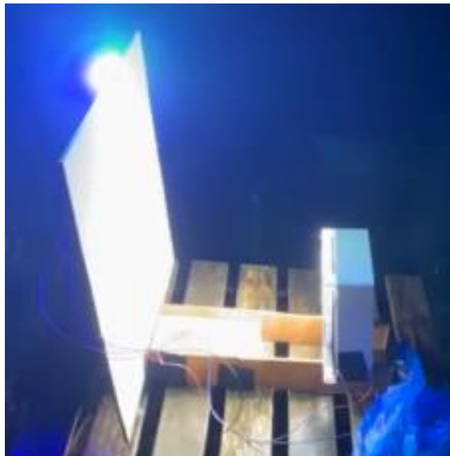
Fig. 4. Prototype operating at night. Landing board with attractive light on the left, main printed circuit board with camera and additional lights on the right. © David Roy, UKCEH.
