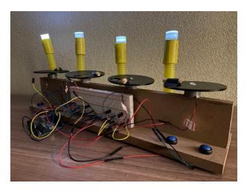
It is worth mentioning that at this stage, no potentiometer was used since the motor needed total power to hit the conduits without stopping. The figure below shows the diagram for the circuit, containing 10K Ohm resistors, a 1A 50V diode, an N-Channel MOSFET 60V 30A, a potentiometer 10K Ohm, a push button, a DC motor, an LED strip with external 12V power source and an Arduino Uno. These are the schematics for one component only and could be repeated to have more components assembled.
