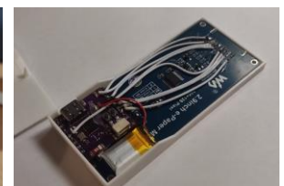
Fig. 2. All of the prototype's components fitted inside the 3D printed case
