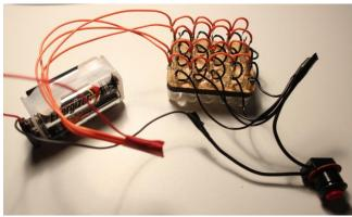
Each LED is connected directly to the photoresistor underneath it, letting more current through as more light is cast onto it. This way, individual pixels can adapt to shadows in real-time, without any processing power.
