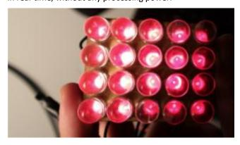
Another other option is take advantage of the LEDs under reverse-bias condition where they can themselves work as light sensors. One could imagine time multiplexing forward and reverse-bias conditions to achieve the functionality on existing displays. Since the light sensitivity tends to
