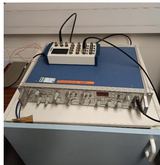
Figure 2: Top : Digitiser, Mid: Axopatch 200B amplifier, Bottom: A faraday cage for sensitive measurements.
