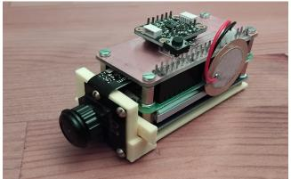
The above image shows the first prototype of Cyclops. The image also shows a button and buzzer that were later added. The image below shows the Lithium Polymer battery from the UPS more clearly.
