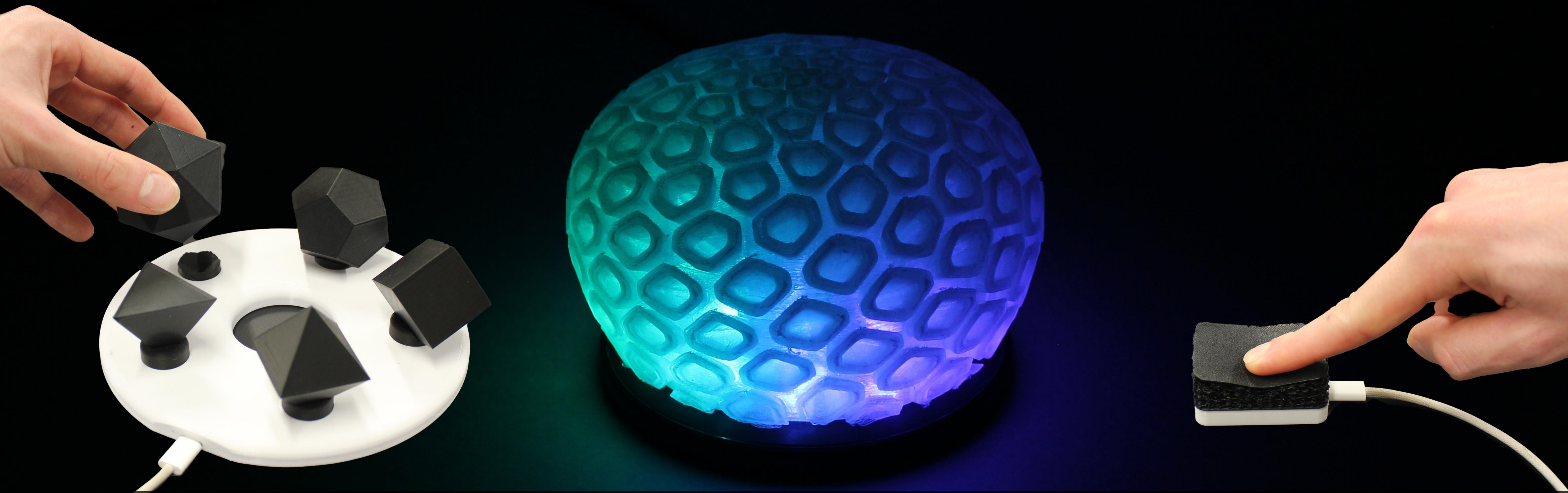
Printegrated prototypes printed on FDM PrusaXL 3D printer, from left to right: Capacitive shape game detects last picked up polyhedron, Wireless smart lamp uses wireless charging and addressable LEDs, Force sensitive haptic input controller
