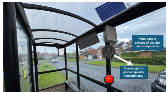
Fig. 2. A mock-up of the smart bus stop system, when delicate components have been covered by weatherproof materials.
