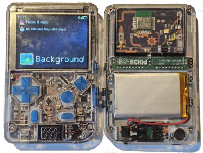
Figure 1 : Device prototype (front & back with inserted cartridge) showing the home screen.
