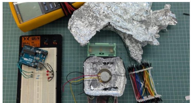
Figure 4: Early aluminium foil shielding experiment investigating non-metal enclosure grounding approaches.
