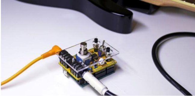
Figure 2: pedalSHIELD UNO by ElectroSmash, an open hardware DSP guitar pedal platform [1].
