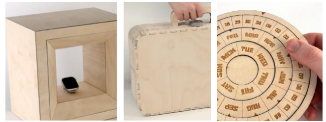
Fig. 7. Our hardware prototype enables new applications for laser cutting, such as objects without visible joints or edges, load-bearing joints such as dovetail joints and cut-in-place mechanisms
