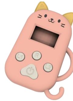
Fig. 1. Figure 1 – KittyGatto 3D rendering showing the cat-shaped enclosure, e-ink display window, physical buttons, and customisable cover.
