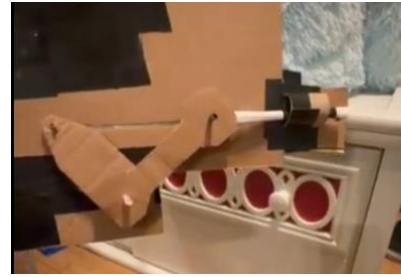
Fig.3. First cardboard prototype of arm retraction method made from cardboard.
